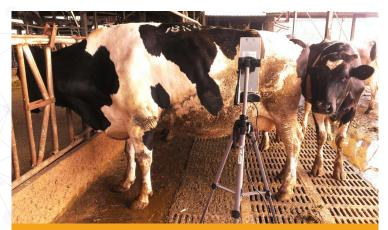
Touch-less monitoring of cow's vital signs using SIL Doppler radar
